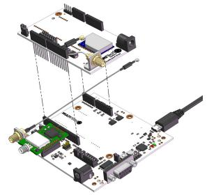
To use an Arduino Shield with an mDot
